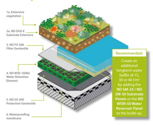
Only when exceeding the storage capacity of the ND WSM-50, due to ongoing rainfalls, the water flows into the ND WSE-100lte Water Retention Element with a retention volume of 95 l/m². The water is stored here temporarily for a period that is set by the calculated flow rate of the ND AFC-200 Adjustable Flow Control
