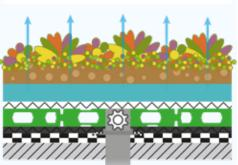
Depending on the intensity and frequency of rainfalls, the main amount of the water will be retained in the vegetation layer and ND WSM-50 Water Reservoir Panel. Only during extreme rainfall, the ND WSE-100lte Water Retention Element will have a retention function. Generally, the water fully contributes to the evaporation and transpiration, enhancing the small water cycles by returning the water to its surroundings.
