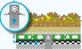
Rain shower occurs and flows through the substrate and is buffered into the ND WSM-50 Water Reservoir Panel until saturation.
