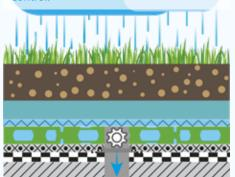
After the rain has stopped the water retained in the ND WSE-100lt Water Retention Element, continues to flow at the set flow rate into the storm water system.
