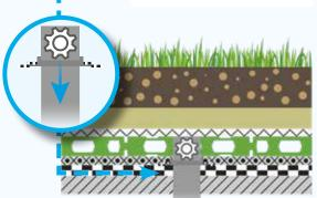
Rain shower occurs and flows through the substrate and is buffered into the ND WSM-50 Water Reservoir Panel until saturation.
