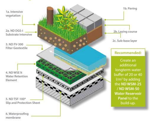
\*In case of an inverted roof construction the ND TSF-100 Protection and Slip Sheet has to be exchanged by the ND 100sv Drainage System.
