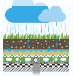
When fully saturated, the ND WSM-50 Water Reservoir Panel buffers 40 l/m<sup>2</sup> water.
