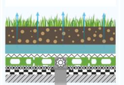
Depending on the intensity and frequency of rainfalls, the main amount of the water will be retained in the vegetation layer and ND WSM-50 Water Reservoir Panel. Only during extreme rainfall, the ND WSE-100lt Water Retention Element will have a retention function. Generally, the water fully contributes to the evaporation and transpiration, enhancing the small water cycles by returning the water to its surroundings.
